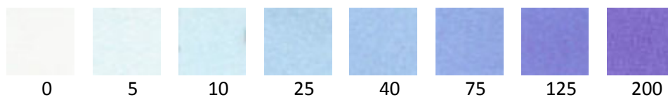
Figure 2: A series of photos of portions of the sensors irradiated with different dosages (rads) of 100 KVP X-ray (batch #0406).
